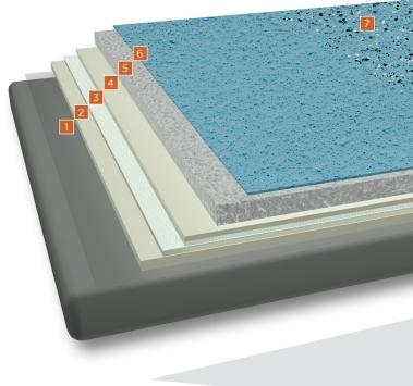
Caltech QC Balcony Plus is a self-finished, thick layer, fully reinforced waterproofing and surfacing system for walkways, balconies and terraces over occupied premises.
