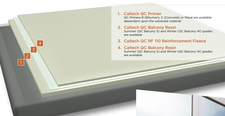
This waterproofing system is a for use beneath coverings and in buried and inverted build-ups for walkways, balconies and terraces - the system is fast curing and fully reinforced.
