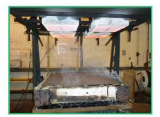
The test methodology measures both the penetration and spread of flame during a specified period, after which the performance rating of the system is determined according to the results observed in the following categories, of which **Broof(14)** is the best, and allows unrestricted use:
