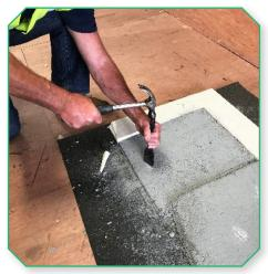
Within approximately 30 minutes from mixing the Monoscreed passed chisel & hammer test.
