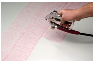
4. Correct application of adhesive
